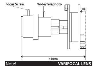
This model contains a varifocal lens that has been pre-focused to a wide angle setting. To adjust to a telephoto mode:
