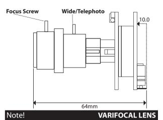
This model contains a varifocal lens that has been pre-focused to a wide angle setting. To adjust to a telephoto mode:
